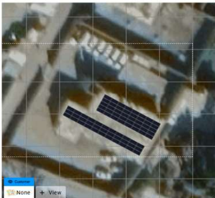
PV layout: 45.99 kWp fit onto the premises.
