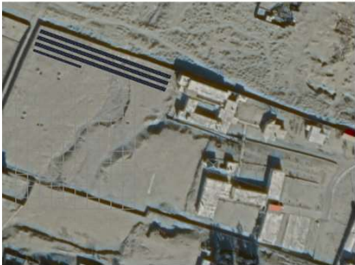
PV layout: 350 kWp fit onto the premises.
