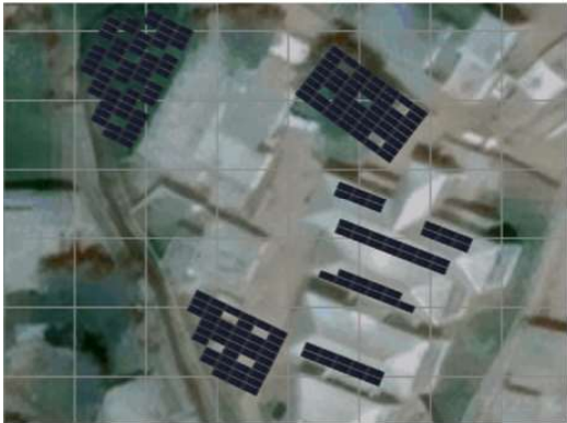
PV layout: 120 kWp fit onto the premises.
