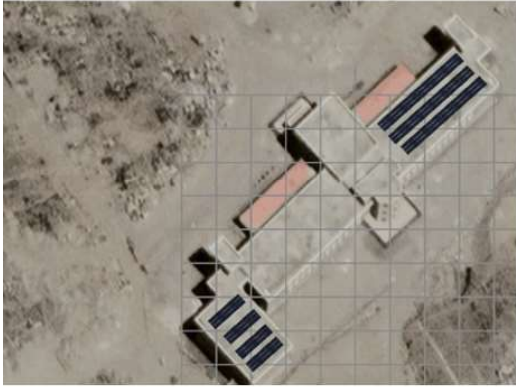
PV layout: 111.5 kWp fit onto the premises.
