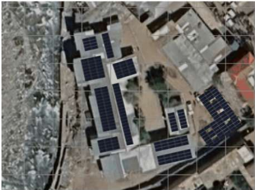
PV layout: 133.6 kWp fit onto the premises.
