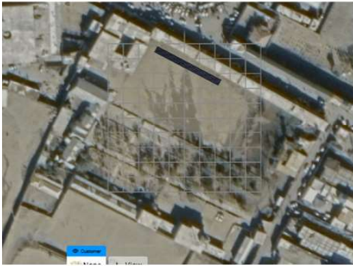
PV layout: 50.4 kWp fit onto the premises.
