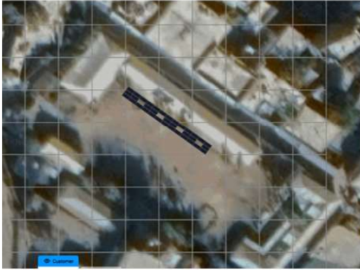
PV layout: 22.05 kWp fit onto the premises.
