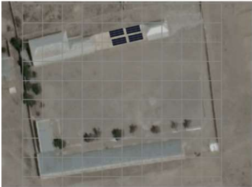
PV layout: 22.68 kWp fit onto the premises.
