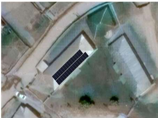
PV layout: 20 kWp fit onto the premises.
