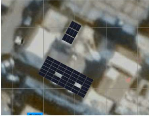
PV layout: 30.87 kWp fit onto the premises.
