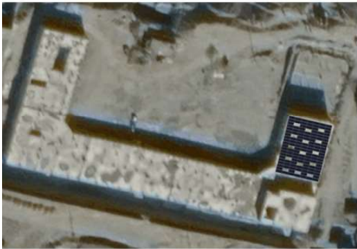
PV layout: 118.4 kWp fit onto the premises.
