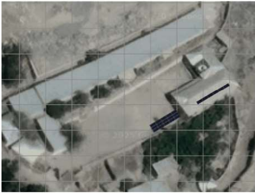
PV layout: 13.23 kWp fit onto the premises.
