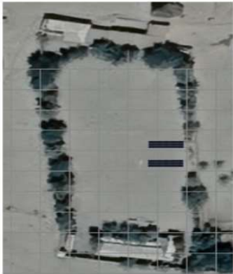
PV layout: 18.9 kWp fit onto the premises.
