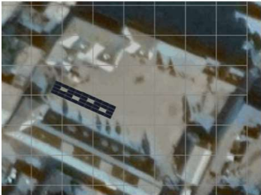
PV layout: 31.5 kWp fit onto the premises.
