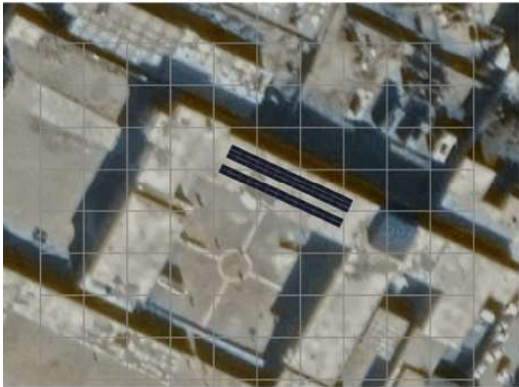
PV layout: 40.95 kWp fit onto the premises.
