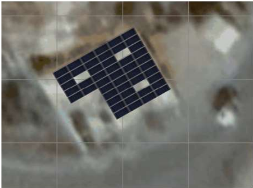
PV layout: 29.61 kWp fit onto the premises.
