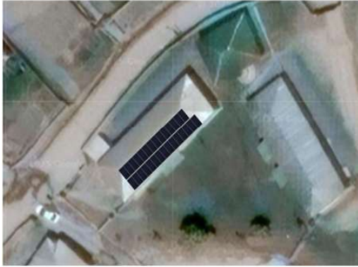
PV layout: 20 kWp fit onto the premises.
